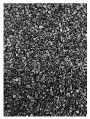
Also, the area of turbulence of Anthracite-Pure is much lesser compared to conventional silica sand media, same goes to the head losses.
