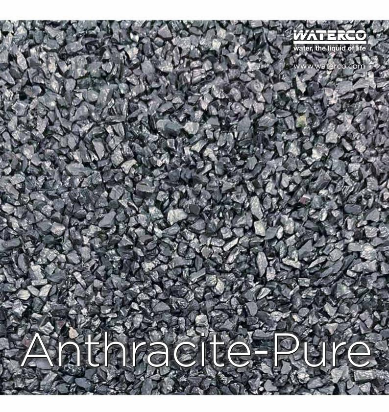
Excellent Filter Media for Multi-Media Application Anthracite-Pure is a top quality coal that consists of hard, durable coal particles to ensure fixed and reliable filtration performance. It is used for turbidity and suspended solid removal. Due to its lighter specific gravity than most of the filter media, Anthracite-Pure is suitable to be paired up as dual or multiple media layer filtration system to enhance the filtration efficiency.
