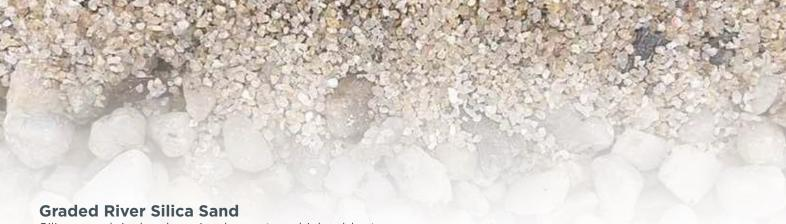
Silica sand is hard grained quartz which able to withstand extreme temperature and high pressure condition. It is an economically feasible filter media for water purification.
