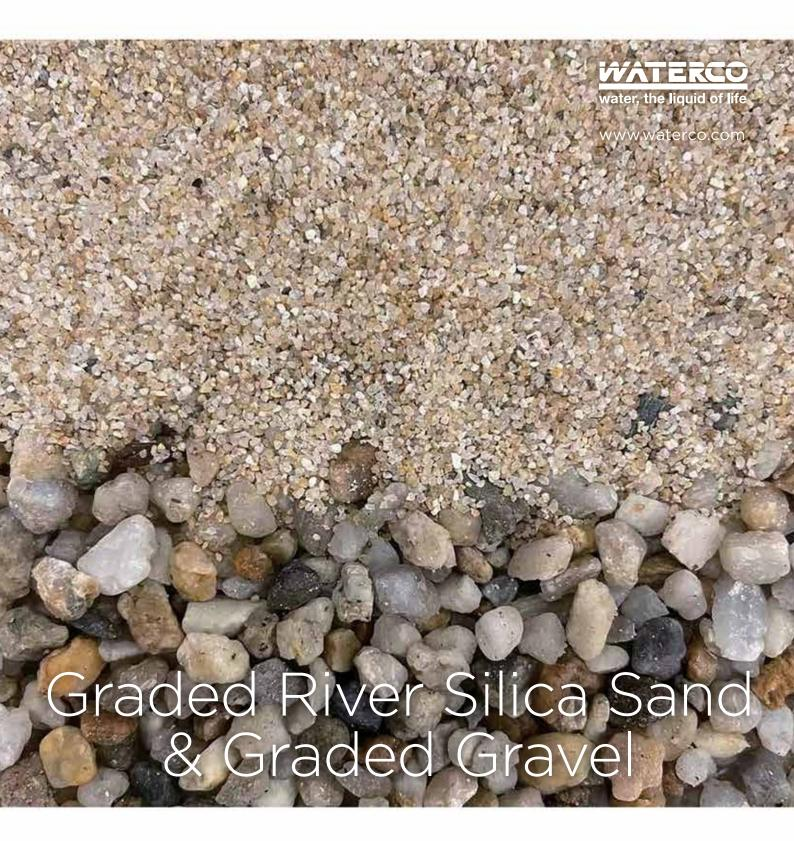
Basic Filter Media for a Filtration System Both silica sand and gravel are carefully selected grade of hard, uniformly graded silica material. They are free from minerals which may precipitate to the systems.
