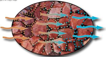
Combining deep bed filtration with ZeoPlus media at a slower filtration rate, is particularly suitable for industrial water treatment plants to achieve superior clean water and ammonia removal.
