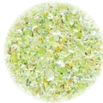
Grade 1 0.5 - 1.0mm (equivalent to Grade 16/30 sand)
