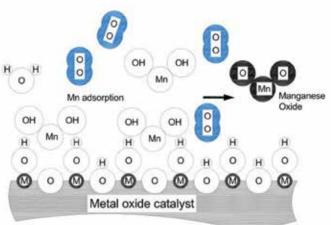
Manganese oxidation at catalytic surface.
